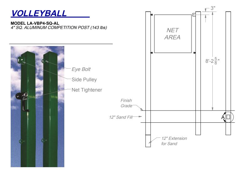
**<u>GENERAL</u>**: Square Volleyball Posts for sprinklers are fabricated using aluminum tubing and are equipped with two (2) fixed eyes on one post and one (1) side pulley, one (1) fixed net tightener and one (1) fixed eye for rope clamp on the other post.
