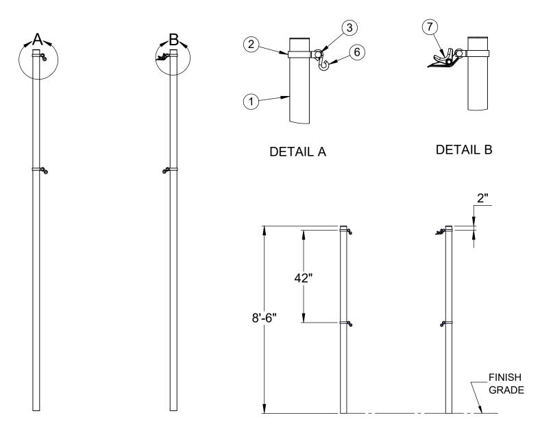
INSTALL THE POSTS IN  $\phi$  18" x 24" DEEP CONCRETE FOOTINGS OR POST SLEEVES. THE TOPS OF THE POSTS ARE 8'-6" ABOVE THE FINISH GRADE.
