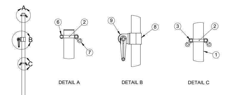
INSTALL THE POST IN A  $\oslash$  18" x 24" DEEP CONCRETE FOOTING OR POST SLEEVE. THE TOP OF THE POST IS 8'-6" ABOVE THE FINISH GRADE.
