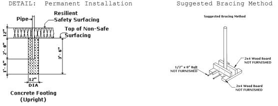
• If resilient surfacing is to be less than 12", then additional pipe should be put in concrete to maintain proper finish grade for equipment.
