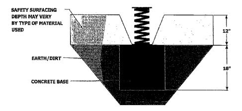
\* If resilient surfacing is to be less than 12", then additional pipe should be put in concrete to maintain proper finish grade for equipment.
