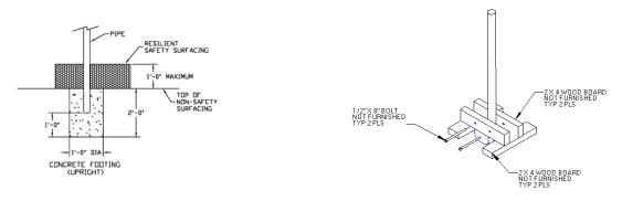
\*If resilient surfacing is to be less than 12", then additional pipe should be put in concrete to maintain proper finish grade for equipment.
