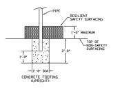
• If resilient surfacing is to be less than 12", then additional pipe should be put in concrete to maintain proper finish grade for equipment.
