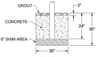
NOTE: FOR SAND INSTALLATION, ADD THE DEPTH OF SAND TO TOTAL.
