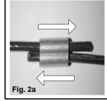
2) When all of the eyelets are threaded, the two ends of the rimlock cable must be secured together. Ensure that there is no slack in the cable at any point. Thread the two cable ends into opposing sides of the supplied aluminum sleeve. (Fig. 2a) Using a large pair of pliers, crimp the sleeve flat at both ends against the rimlock cable. (Fig. 2b) This must be crimped well to prevent the cable from slipping.
