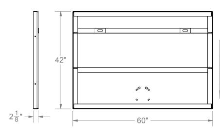
The Model 19 is fabricated from a single sheet of heavy duty aluminum and heavily reinforced around the perimeter and interior with 2" x 2" x 3/16" aluminum angle and powder coated white after fabrication.
