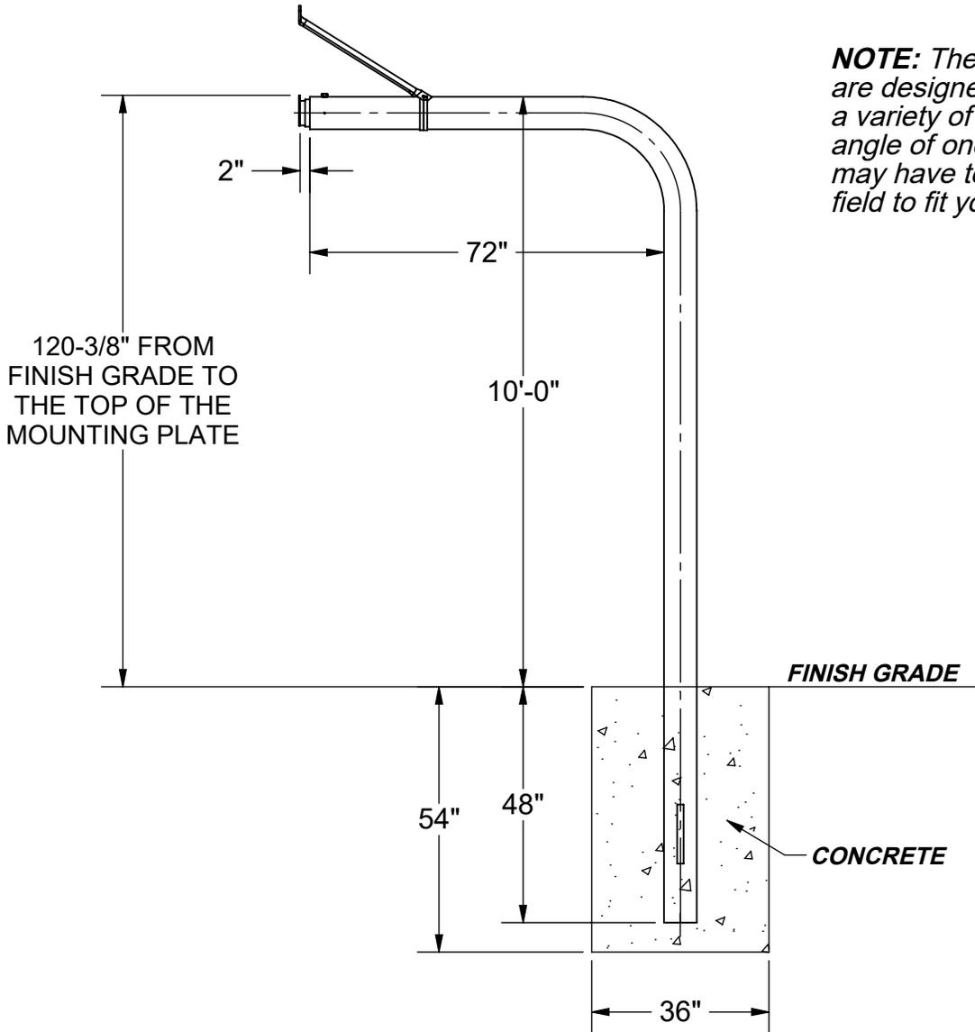
**NOTE:** The backboard braces are designed to accommodate a variety of backboards. The angle of one end of the brace may have to be adjusted in the field to fit your backboard.
