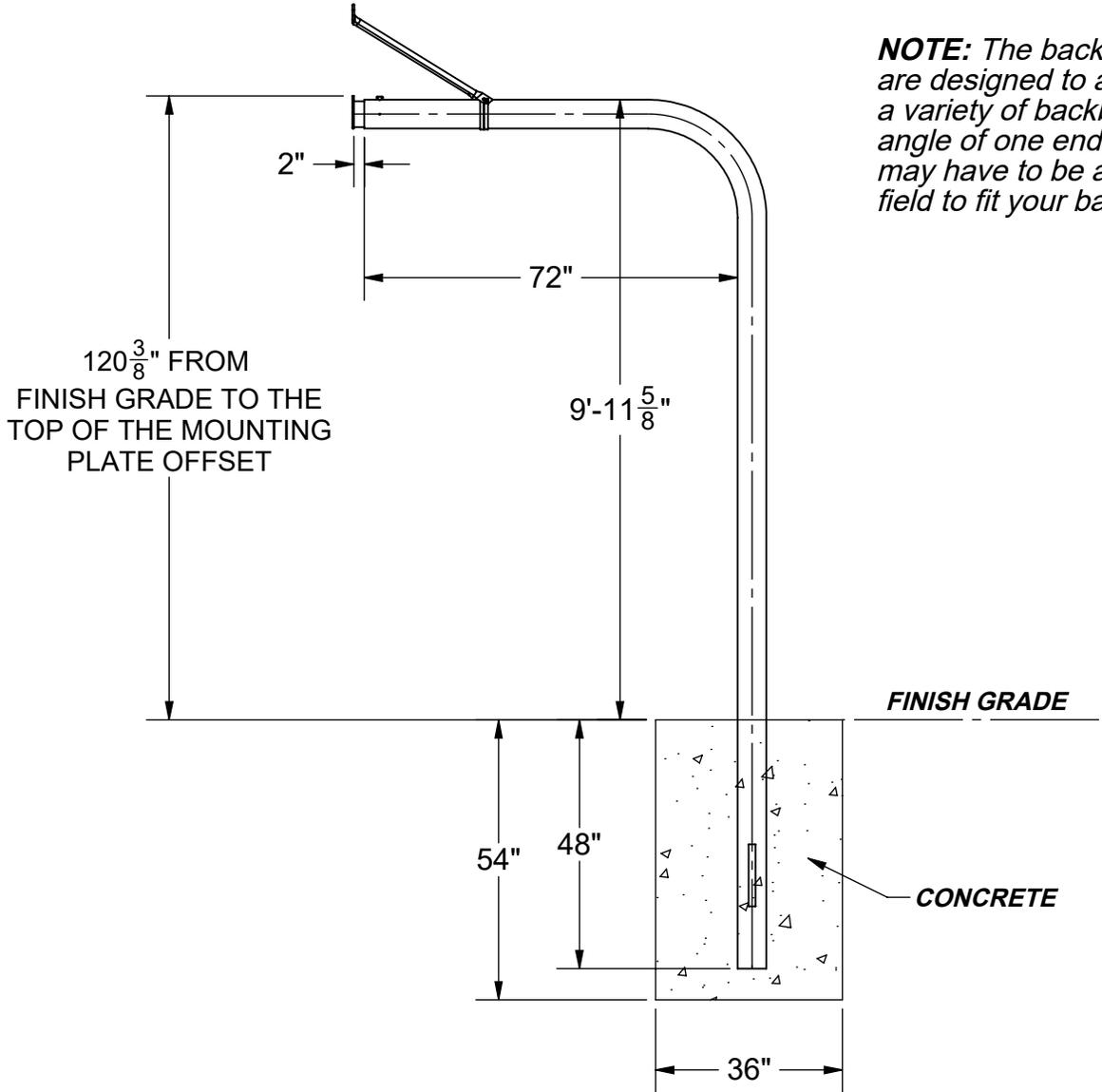
**NOTE:** The backboard braces are designed to accommodate a variety of backboards. The angle of one end of the brace may have to be adjusted in the field to fit your backboard.
