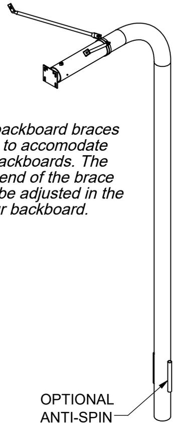
**NOTE:** The backboard braces are designed to accommodate a variety of backboards. The angle of one end of the brace may have to be adjusted in the field to fit your backboard.
